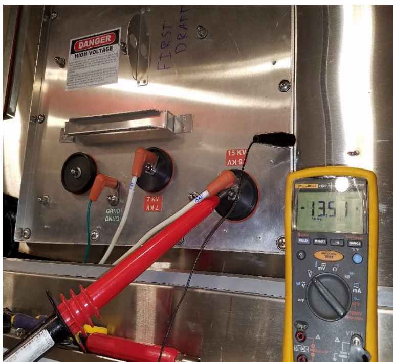
Figure 4-9-1,2 Setting the ESP cell Voltage
