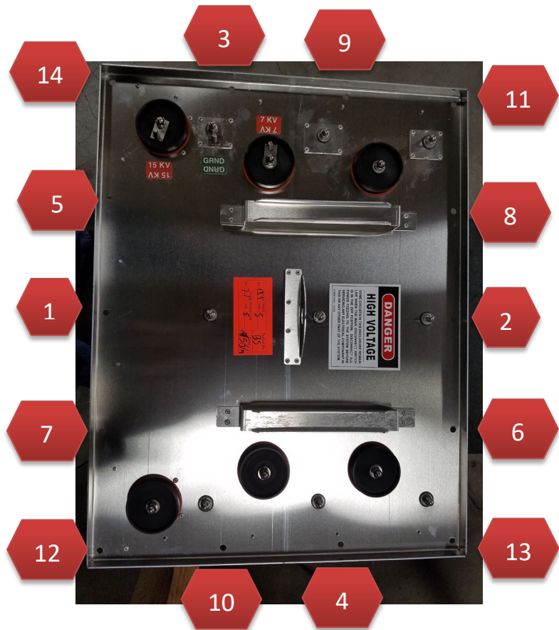
Figure 3-9-1 ESP Cell Bolt Tightening Schedule – Re-installation
