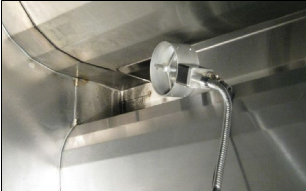
Figure 6-3-1 2 3/4" Rotating Vane Anemometer Sensing Head at Air Inlet Slot
