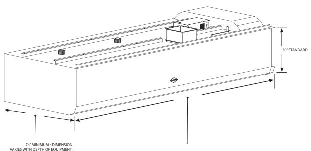
6'- 1" MINIMUM UNIT LENGTH. FOR GREATHER LENGTH, JOIN TWO OR MORE SECTIONS TOGETHER. ALLOW 6" MINIMUM OVERHANG AT EACH END. IF CHARBROILER IS AT END, OVERHANG 12".
