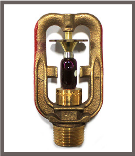
G. 16402 - 325 DEGREE, 160° SPRAY ANGLE, 1/4" ORIFICE
