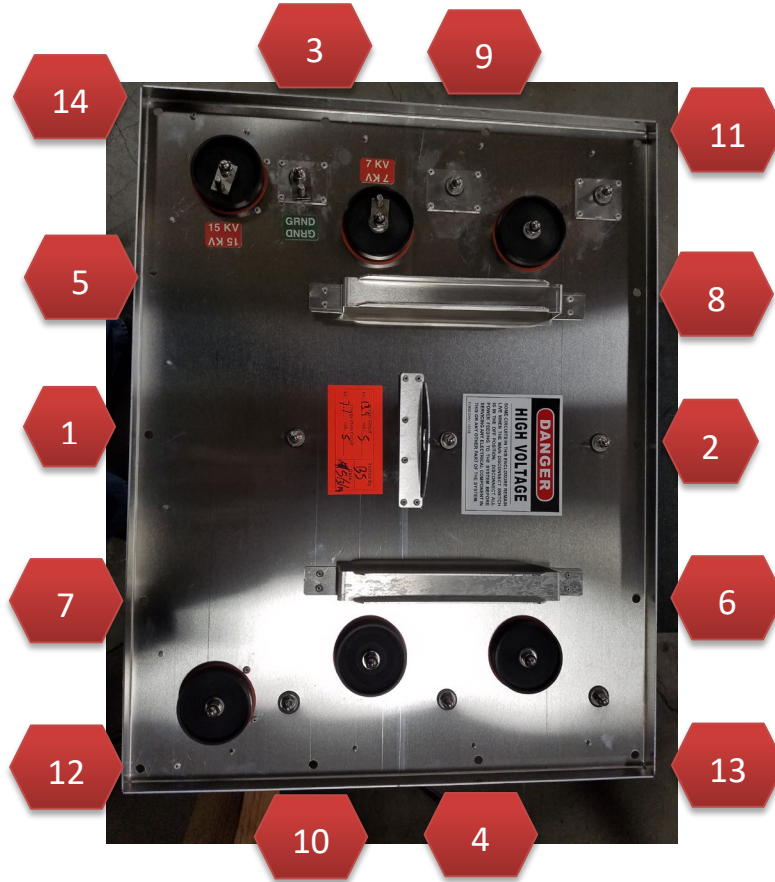
Figure 3-9-1 ESP Cell Bolt Tightening Schedule – Re-installation
