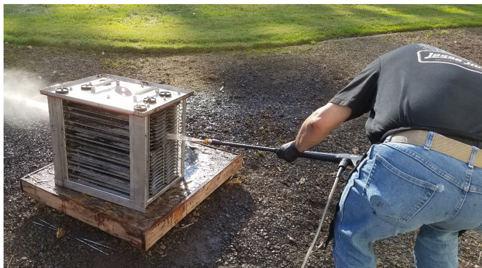
Figure 3-8-1 ESP Cell "Cautious Pressure Washing"
